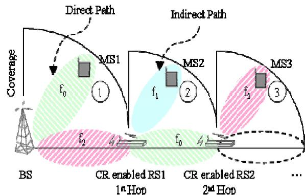
Figure 1. CR based multi-hop cell architecture
