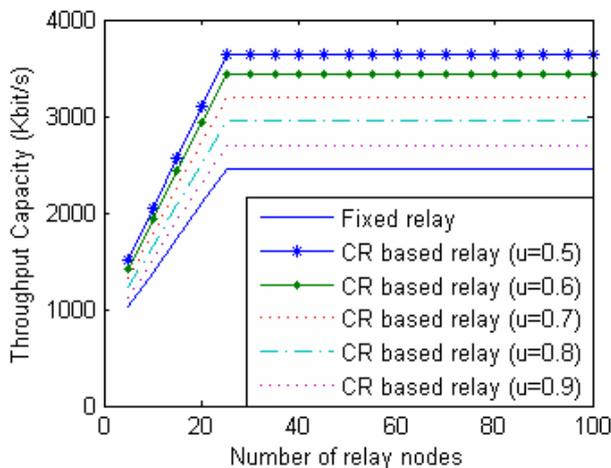
Figure 2. The throughput capacity of the proposed system varying utilization factor
