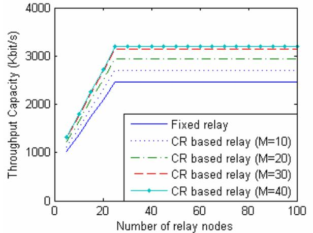
Figure 3. The throughput capacity of the proposed system varying number of CRs
